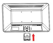
3. Unpack the base and attach to stand as shown.
